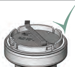
Seal in the groove: correct
