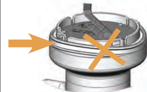
Seal not in the groove: NOT correct
